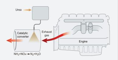
The principle for Scania SCR system
